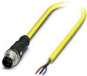
Sensor/Actuator cable, 3-position, TPE, yellow RAL 1021, Plug straight M12 SPEEDCON, A-coded, on free cable end, Cable length: 5 m
